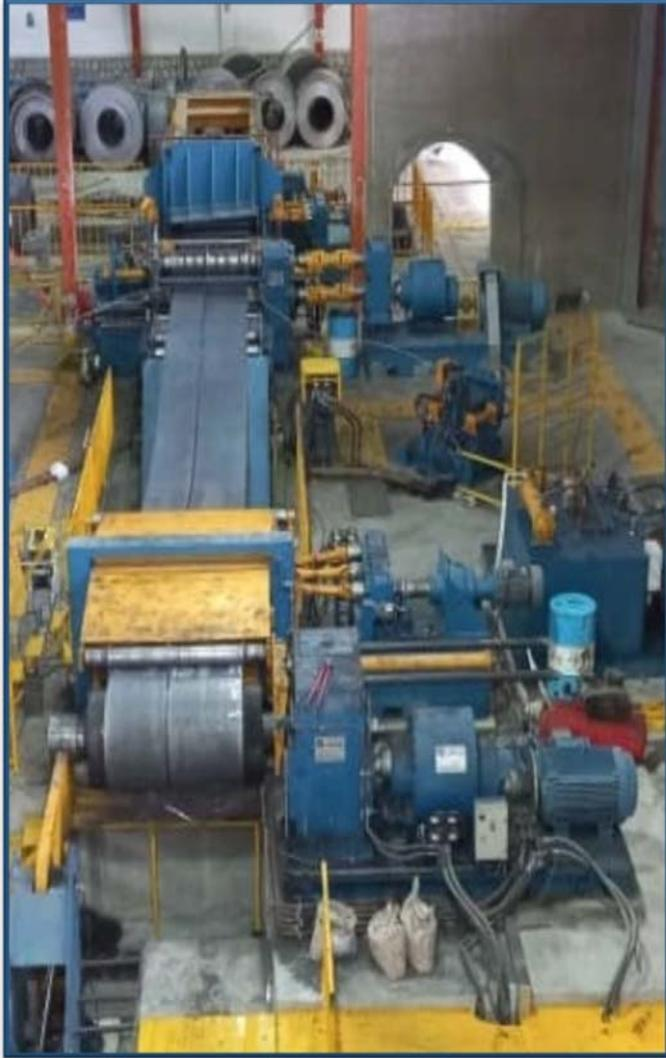
20 tons, 1550 mm width, 4 mm sheet thickness
